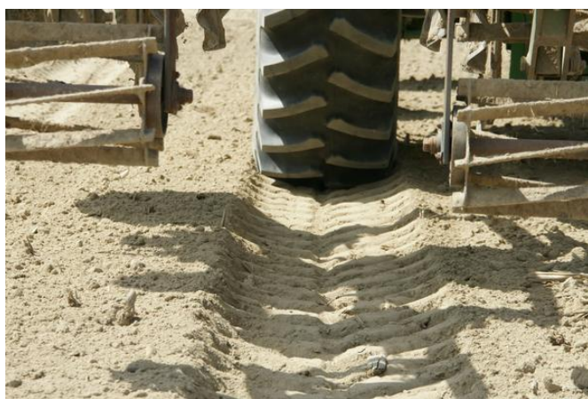
Farm equipment tires causing soil compaction. Photo from NC State Extension.
